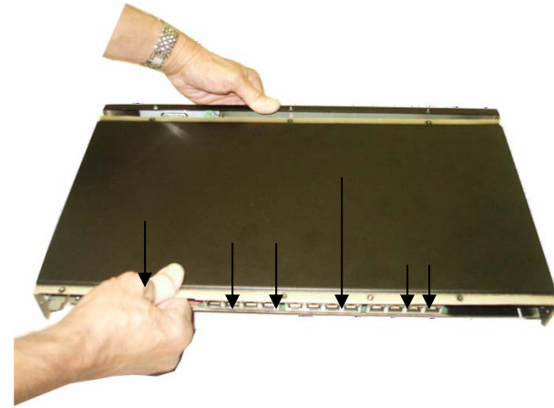
Fig 3.5.1b: Pulling out the top cover from the chassis base
